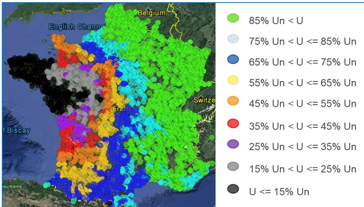
Figure 6. Example of propagation of the fault in the 400kV western part of the French transmission system
