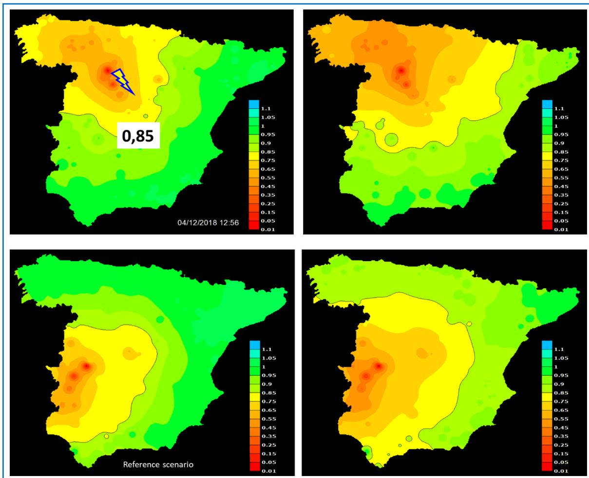
Figure 7. The effect of a fault in the transmission system and its impact in terms of voltage dip across the electrical network during two different faults, affecting most of the Spanish electrical system.
